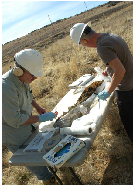
Workers opening cores from a soil boring to examine and sample.
